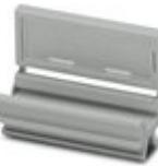
Group marking label, snaps onto terminal center for screw, spring-cage and quick connection terminal blocks, labeled with ESL 26x6 mm or EST 25x6 mm, in the foot part with Zack marker strip, length: 29 mm
