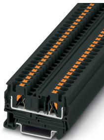
Feed-through terminal block, nom. voltage: 800 V, nominal current: 32 A, connection method: Push-in connection, 1 level, Rated cross section: 4 mm<sup>2</sup>, cross section: 0.2 mm<sup>2</sup> - 6 mm<sup>2</sup>, mounting type: NS 35/7,5, NS 35/15, color: black
