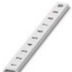
Zack Marker strip, flat, Strip, white, labeled, printed horizontally: consecutive numbers 1 ... 10, 11 ... 20, etc. up to 91 ... 100, mounting type: snap into flat marker groove, for terminal block width: 6.2 mm, lettering field size: 5.15 x 6.15 mm, Number of individual labels: 10
