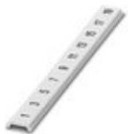
Zack Marker strip, flat, Strip, white, labeled, printed horizontally: Odd numbers 1 - 19, 21 - 39, etc. up to 81 - 99, mounting type: snap into flat marker groove, for terminal block width: 6.2 mm, lettering field size: 5.15 x 6.15 mm, Number of individual labels: 10
