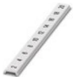
Zack Marker strip, flat, Strip, white, labeled, printed horizontally: consecutive even numbers 2 ... 20, 22 ... 40, etc. up to 82 ... 100, mounting type: snap into flat marker groove, for terminal block width: 6.2 mm, lettering field size: 5.15 x 6.15 mm, Number of individual labels: 10
